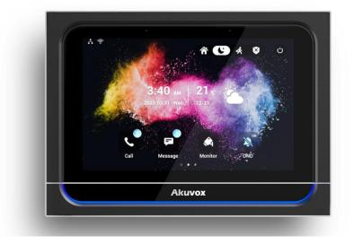
X933 series is an Android SIP-based with a smooth touch-screen indoor monitor. It can be connected with the Akuvox door phone for audio/video communication, unlocking, and monitoring.Residents can communicate with visitors via audio/video call, and it supports unlocking the door remotely. It is more convenient and safer for residents to check the visitor's identity through its video preview function. X933 series are often applied to scenarios such as villas, apartments, and buildings.
