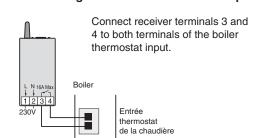
If necessary, remove the shunt (electric wire) connecting the two thermostat input terminals.
