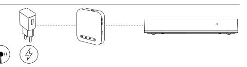
In the event of a power failure, the device will automatically switch to a backup source. After power network outage the HubPowerbank can provide power and internet connection up to 12 hours.
