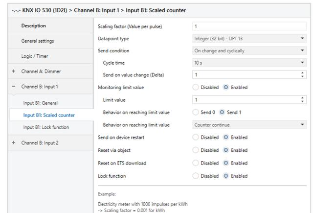
This counter can be used to count values on input impulses, where an integer value or a floating-point value can be selected as a counter variable. With this function, e.g. Electrical energy can be counted directly and sent to the bus via an object.
