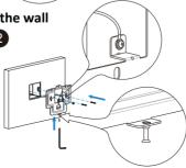
Twist M3x10.5 screw into the bottom hole of the wall bracket until the tail of which align to the edge. Then fix the wall bracket on the wall with two/four M4x30 screws. If there is a ground wire to be connected , use M3x6 screw to fix it on the wall bracket.
