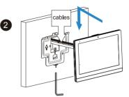
Connect the cables to device.
